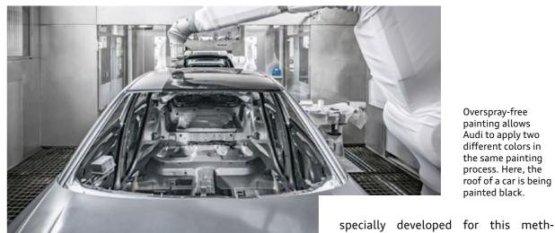
Overspray-free painting allows Audi to apply two different colors in the same painting process. Here, the roof of a car is being painted black.
